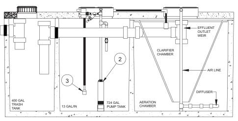
The heart of the system is a NSF certified treatment works producing 10/10 effluent housed in a single concrete tank.
