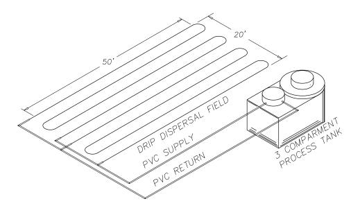
changed. The effluent dispersal field uses inexpensive polyethylene tubing incorporating pressure balanced emitters for uniform dispersal. During the dosing cycle the tubing is continuously flushed, with any particulate being returned to the pump tank A typical drain field can be as little as 1000 square feet.
